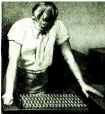
Here we have the new Lynch resistors undergoing "flash" test. (No. 254)
