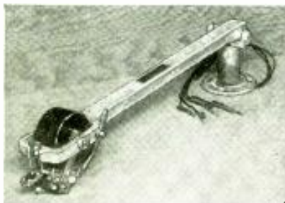
Special Universal recording head for the more "ambitious" short-wave fan; this head actually cuts the groove in the record, a lead-screw propelling it across the disc.
