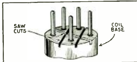
The trick shown above will considerably reduce high frequency losses in plug-in coil forms.
