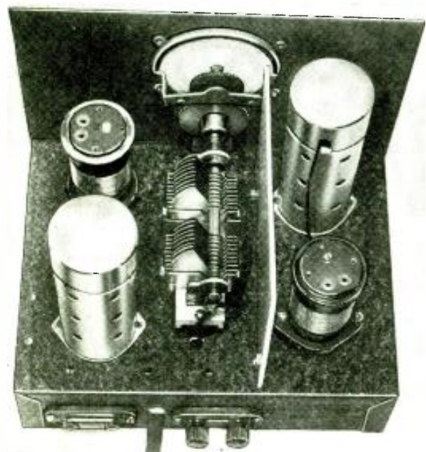
Left—Rear view of the "Economy 3" showing the placement of parts. Right—Underneath view—note that one of the tubes has been mounted under the chassis in order to simplify wiring and make the receiver more compact.
