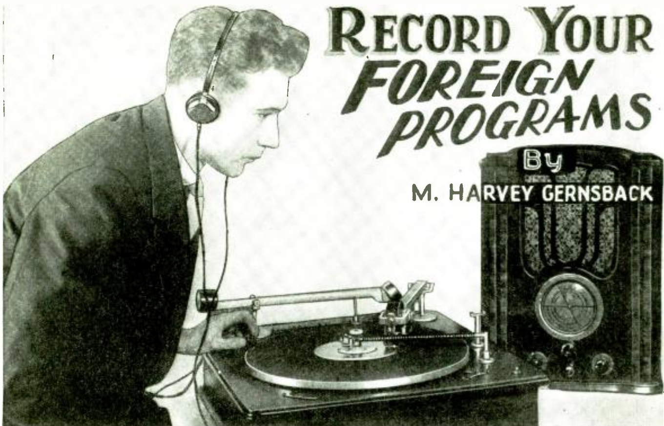
The recording machine shown in the center of the photo is that designed and built by the Universal Microphone Company and handles full-sized records. The lead-screw propels the recording head across the record so that it can cut the grooves as it moves along. The magnetic pick-up is shown at the rear of the machine and the headphones serve as a monitor.
